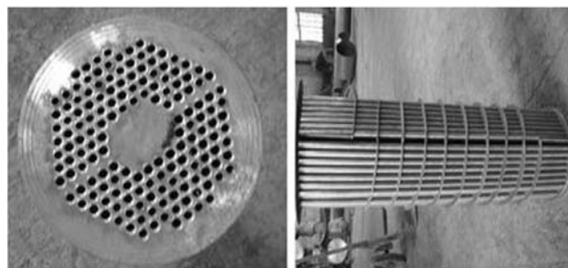
Fig. 5 Tube bundle of the STHX with continuous helical baffles (for CS and CM): (a) end view and (b) side view
